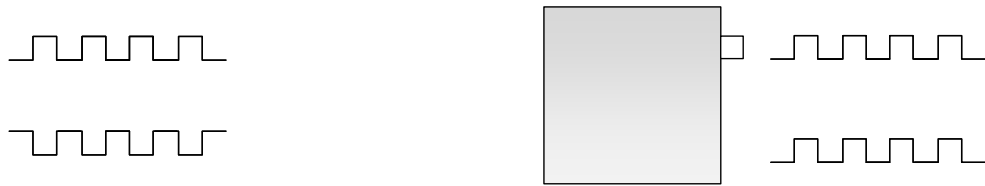
Figure 3.5. Integrated 1:2 CMOS Buffer Supports In-Phase or Complementary Outputs
